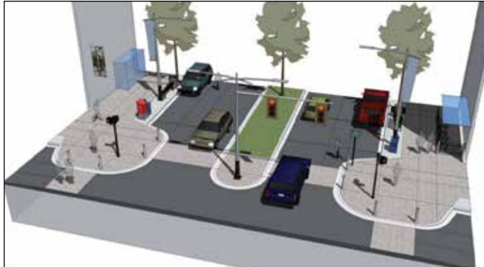
Figure D21: This image shows how the use of curb extensions, a centre median and on-street parking enhance a pedestrian street.
