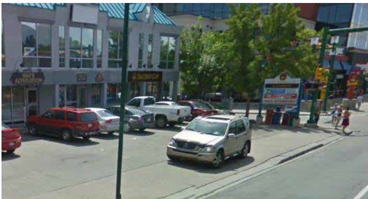
Figure D32: This image demonstrates unacceptable streetscape design further south on the same street: A commercial building with a parking area between the building and sidewalk creates conflict between automobiles and pedestrian movement.
