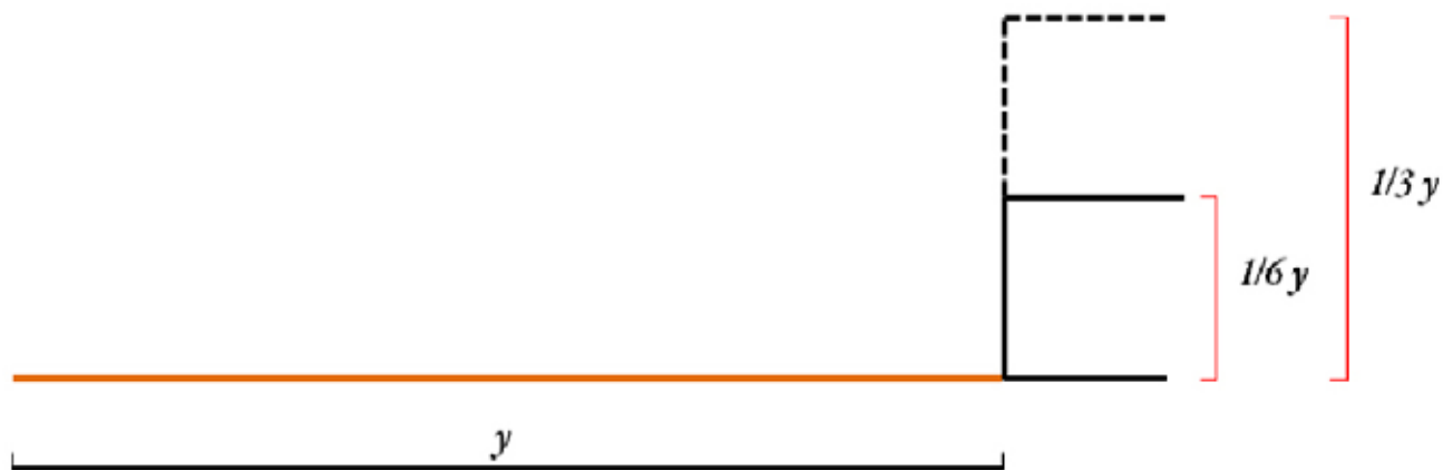
Figure D40: A simple schematic showing the range of building heights deemed appropriate in a Neighbourhood Activity Centre. In this case, ideal building heights range from one-sixth to one-third the width of y , which represents the width of a street (including sidewalk and boulevard), amenity space or both.
