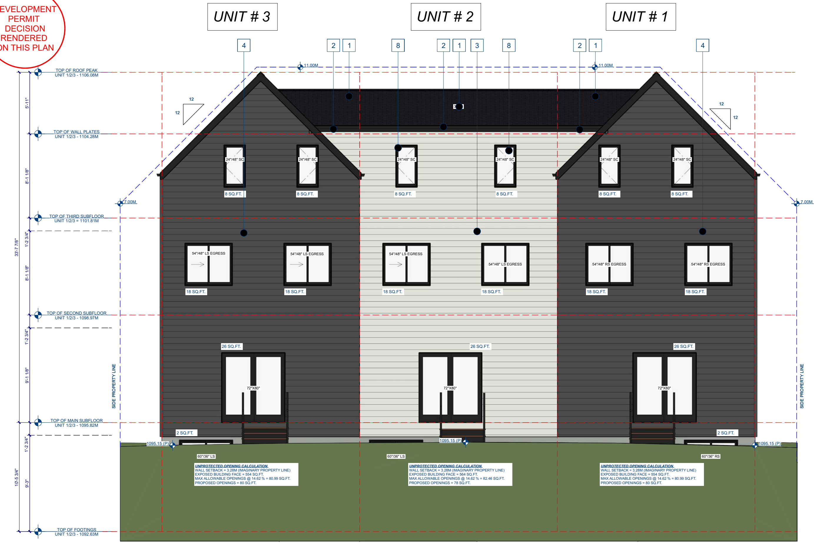
1 REAR ELEVATION - FRONT BUILDING A6 SCALE = 3/16" = 1'-0"
