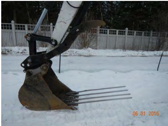
Photo 3-50: Forks welded to a bucket to create planting holes in timber crib wall backfill for a site on the Elbow River
