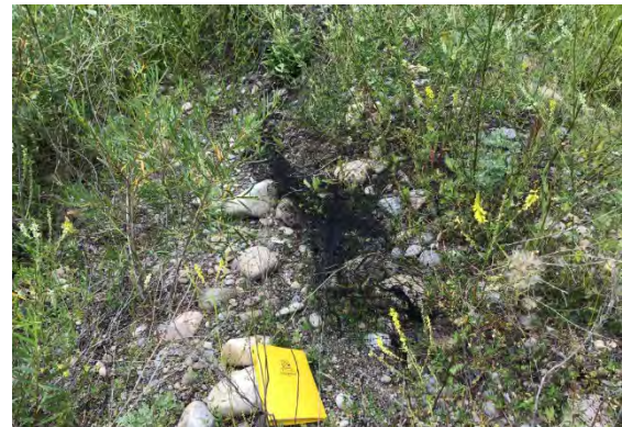
Photo 3-15: Example of the remains of synthetic erosion control matting that was installed in 2008 and observed in 2020
