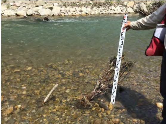
Photo 3-28: Example of container plant in an eroded section of side channel on the Bow River in 2018 and assessed in 2019
