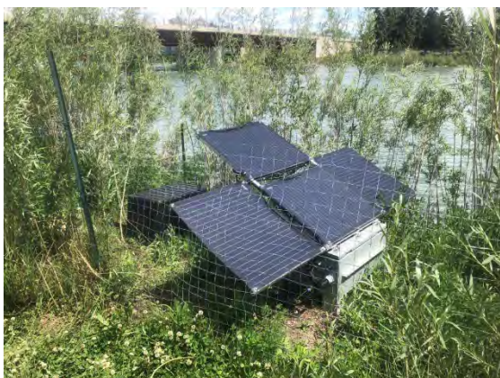
Photo 3-52: Example of a solar powered irrigation system on a bioengineering site on the Bow River
