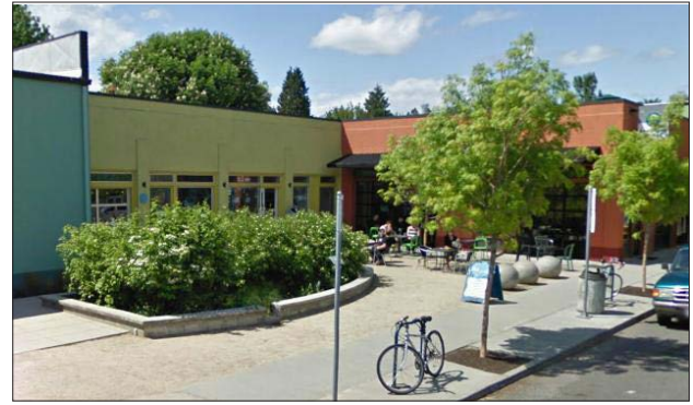
Figure C24: This shows a rain garden designed to capture rain water from adjacent rooftops. It has been incorporated in such a way as to delineate the private realm from the public realm and provide enclosure to a patio.
