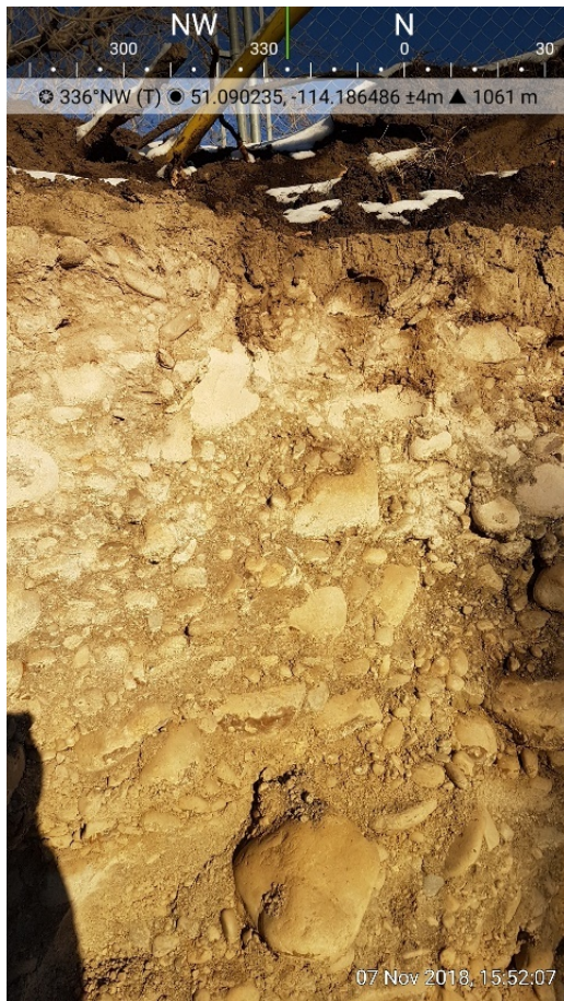
Figure III-5.1 Photograph of Excavation at 6750 Crescent NW showing Alluvial Sand and Gravel Unit
