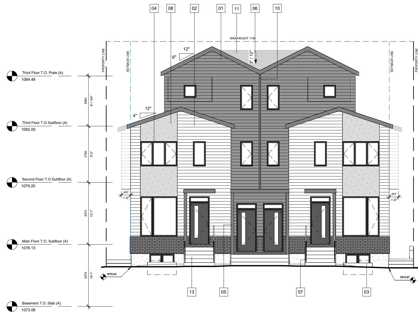
1 BUILDING A @ FRONT (SOUTH) ELEVATION 3/16" = 1'-0"
